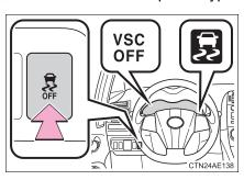
Press and hold the button for more than 3 seconds while the vehicle is stopped to turn off TRC and VSC.
