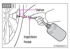
Connect the injection hose to the valve.
