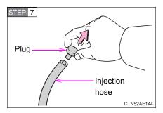
Remove the plug from the injection hose.
