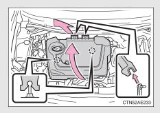
Raise the front of the engine cover to detach it from the clips and then pull the cover to detach it from the brackets on the rear bar as shown in the illustration.
