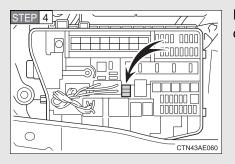
Remove the fuse with the pullout tool.
