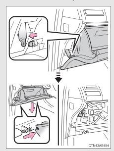
Open the glove box and slide it off the damper, lifting it to disconnect the claws at the bottom.
