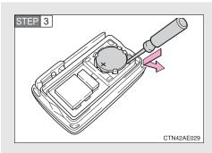
Remove the depleted battery.
