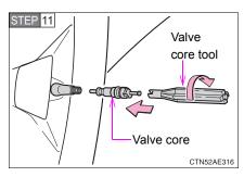
Remove the injection hose from the valve and screw the valve core in the valve securely by turning it clockwise with the valve core tool.
