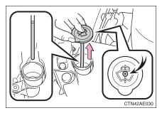
If the fluid level is extremely low add washer fluid.
