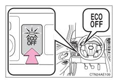
Press the "ECO OFF" switch to disable the Stop & Start system.
