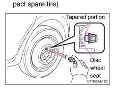
Tighten the nuts until the tapered portion comes into loose contact with the disc wheel seat.
