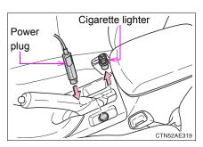
Vehicles with a cigarette lighter: Remove the cigarette lighter and insert the compressor power plug into the hole.
