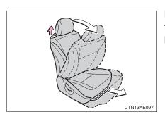
Lift the walk-in lever and move the seat as far forward as possible.
