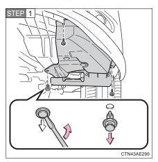
Remove the fender liner bolts and clip.
