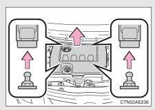
Raise the rear of the engine cover to remove the two rear clips, and then raise the front of the engine cover to remove the two front clips.
