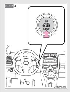
Press the "ENGINE START STOP" switch.
