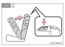
Fold the seatback while pressing the seatback angle button. Return the seatback and secure it at the first lock position.
