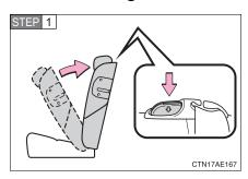
Fold the seatback while pressing the seatback angle button. Return the seatback and secure it at the first lock position.  $(\rightarrow P. 68)$
