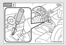
Press the shift lock override button with a flathead screwdriver or equivalent.
