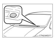
Headlight control sensor is located on the driver's side.
