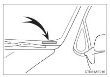
On right-hand drive vehicles, this number is also stamped on the top left of the instrument panel.
