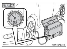
Read the inflation pressure on the pressure gauge.
