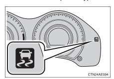
If the vehicle is in danger of slipping or the front wheels spin, the indicator flashes to indicate that the VSC/TRC systems have been engaged.
