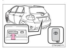
Press the button to unlock the doors.
