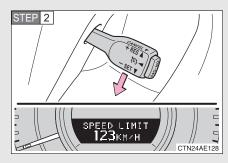
Accelerate or decelerate to the desired speed and push the lever down to set the desired maximum speed.
