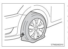
A tire should only to be repaired if the damage is caused by a nail or screw passing through the tire tread. Perform the repair with the nail or screw that has punctured the tire positioned at the bottom, in contact with the ground.
