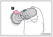
Wash/wipe operationWipers operate automatically.
