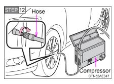
Connect the air compressor hose by threading it on the valve.
