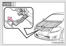
Push the hood catch to the left and lift the hood.
