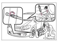
Vehicles with a cigarette lighter: After driving about 5 km (3 miles) or 10 minutes, pull your vehicle over in a safe place and reconnect the compressor.
