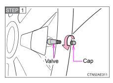
Position the nail or screw that has punctured the tire at the bottom, in contact with the ground. Remove the cap from the valve.
