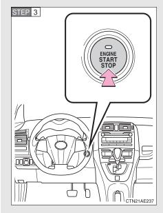
Press the "ENGINE START STOP" switch.
