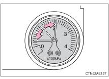
If the pressure is 130 kPa (1.3 kgf/cm<sup>2</sup> or bar, 18 psi) or above, fill the tire with air using the compressor until the specified inflation pressure is reached.
