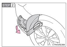
Remove the fender liner.
