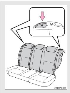
Press the button down until the lock is completely released to adjust the seat-back angle.
