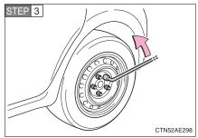
Slightly loosen the wheel nuts (one turn).
