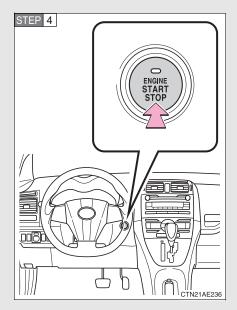
Press the "ENGINE START STOP" switch.
