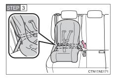
Run the seat belt through the child seat and insert the plate into the buckle. Make sure that the belt is not twisted. Keep the lap portion of the belt tight.
