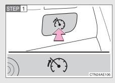
Turn the speed limiter switch on.
