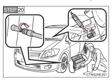
Vehicles with a power outlet: After driving about 5 km (3 miles) or 10 minutes, pull your vehicle over in a safe place and reconnect the compressor.
