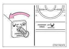
Insert the key into the cylinder and rotate to the "OFF" position.
