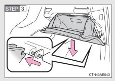
Lift the glove box to disconnect the claws at the bottom and remove it.
