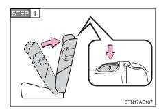
Fold the seatback while pressing the seatback angle button. Return the seatback and secure it at the first lock position.
