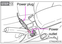
Vehicles with a power outlet: Connect the compressor power plug to the power outlet.
