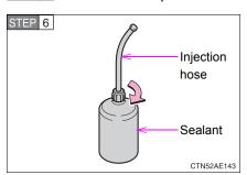
Connect the injection hose by screwing onto the sealant. As it is screwed in, the aluminum seal on the bottle will be torn.
