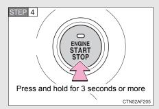
Vehicles with a smart entry & start system: Stop the engine by pressing and holding the "ENGINE START switch for 3 consecutive seconds or more.
