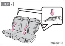
Fold the seatback down while pushing the seatback angle adjustment button.
