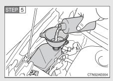
Add engine coolant if necessary.
