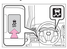
Quickly press and release the button to turn off TRC.
