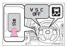
Press and hold the button for more than 3 seconds while the vehicle is stopped to turn off TRC and VSC.
