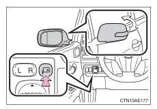
Press the switch to fold the mirrors.
