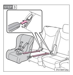
Check the positions of the exclusive fixing bars, and install the child restraint system to the seat.
