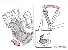
Adjust the second seat forward so that it does not interfere with the child restraint system.
