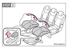
Pull the seatback angle adjustment lever to flatten the seatback.
