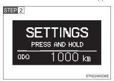
Press and hold the "DISP" switch to enter the adjustment mode.
