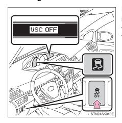
Push and hold the button for more than 3 seconds while the vehicle is stopped to turn off TRC and VSC+.
