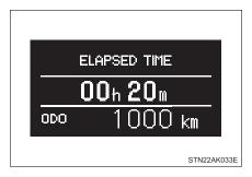
Displays the elapsed time since the engine was started or since the function was last reset.
