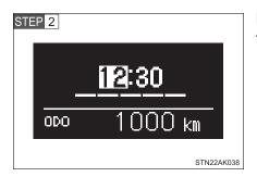
Press the "DISP" switch to adjust the hours.
