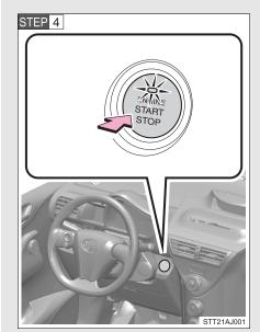
Press the "ENGINE START STOP" switch.
