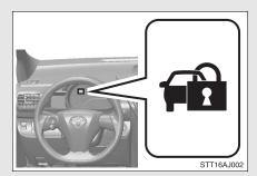
Close the doors, back door and hood, and lock all the doors using the entry function (vehicles with smart entry & start system) or wireless remote control. The system will be set automatically after 30 seconds.
