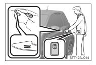
If the doors cannot be locked by touching the lock sensor provided on the upper edge of a door handle, simultaneously touch the lock sensors provided on the upper and lower edges of the door handle.
