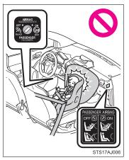
Never use a rear-facing child restraint system on the front passenger seat when the airbag manual on-off switch is ON. (→P. 159)
