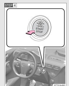
Press the "ENGINE START STOP" switch.
