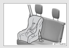
An ELR belt requires a locking clip to install a child restraint system.
