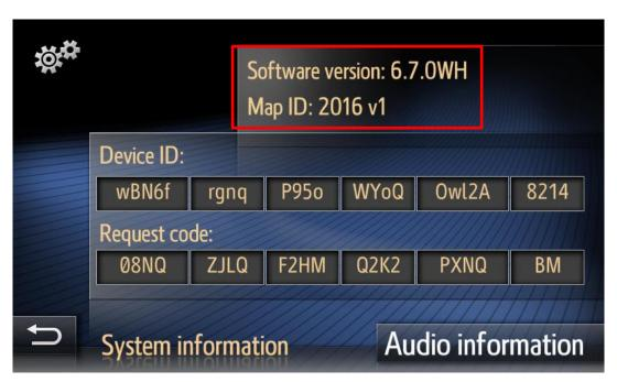
If the software version is lower than 4.4.0, the map is not configurable. The full EU map is always installed. Performing a map update will give the possibility to reconfigure the map.
